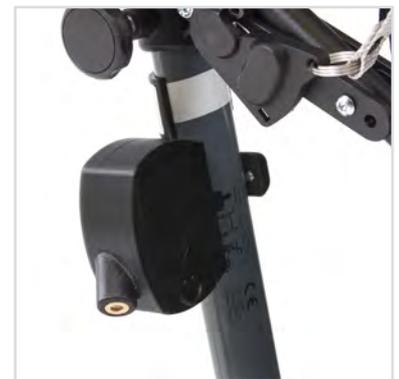
**The laser light unit** receives wireless signals from the switch on the handle and produces a green laser light which shows as a line between the rear wheels of the rollator. After 15 seconds the light is automatically turned off. If desired this can be adjusted. The green laser light is known to be six times more visible than red.
